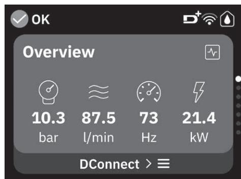
The Dashboard screen displays certain parameters depending on the following conditions: whether or not there is a flow meter, and whether or not the pump belongs to a group. On the main screen, the various parameters are displayed depending on the following conditions: whether or not there is a flow meter, and whether or not the pump belongs to a group. The parameters that can be displayed are as follows:
