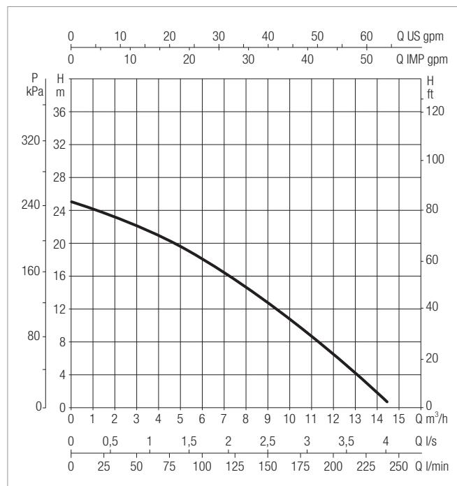
The performance curves are based on kinematic viscosity values = 1 mm<sup>2</sup>/s and density equal to 1000 kg/m<sup>3</sup>. Curve tolerance according to ISO 9906.
